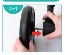
How to disassemble the rear wheels
