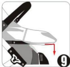
You can adjust the sitting posture and sleeping posture under different conditions by pulling the foot pallet forward and releasing it downward at the same time.
