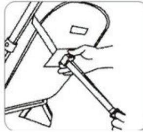
**Backrest Height Adjustment:** When one hand holds the lower end of the adjustment buckle, the other hand holds two sides of the adjustment buckle. Switch tightly to make the buckle relaxed and then push the adjustment buckle up and down, adjust to the appropriate angle and then open the adjusting buckle which is in a locked state. The operation is complete.
