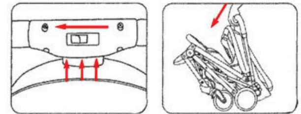
**Closing Operation:** Hold the lock piece on the push handle by hand, press the button of the second lock on the right thumb and at the same time, the other four fingers hold the button of closing the car upwards, push to the front and bottom of the car and the car will fall down and close, hang up the side car hook and the process is complete.
