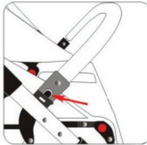
**Handrail Operation:** For the convenience of the baby in and out, this car is designed for disassembling the handrail, press the buttons on the left and right sides, and then pull out the handrail with a little strength, then it can be disassembled. On the contrary, insert it directly to make the button pop up, and do not pull it out with force that is, the installation is successful.
