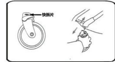
Assemble the front wheel shaft. Turn the front wheel slightly to check whether the rotation is flexible. If it cannot be pulled out, it is qualified. When removing, pull out the bottom of the front wheel axle sleeve.
