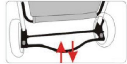
**Rear Wheel Brake Operation:** After gently stepping down the rear wheel brake lever, the car is in a brake state and cannot be carried out. Lift up the brake lever to release the brake state.
