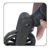
3. Front wheel removal press and hold the gray dot button to remove the front wheel.
