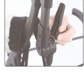
5. The bracket grooves are alligned with the grooves on the frame and pushed inward untill its in the bottom completely.
