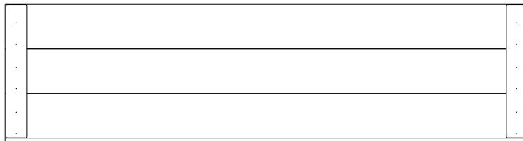
RP6 | ROOF PANEL - W2A02627 (4) | 1 5/8"x15 5/8"x59" (42x396x1499)
